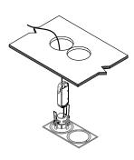
3 Connect mains from ceiling to driver (as per luminaire instructions) then fold luminaire springs up and pass driver and luminaire through ceiling hole
