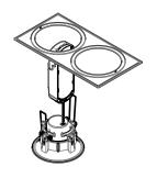
2 Fold luminaire springs up and pass driver and luminaire through plate
